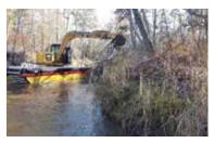
Amphibious equipment removing vegetative debris from stream channel
