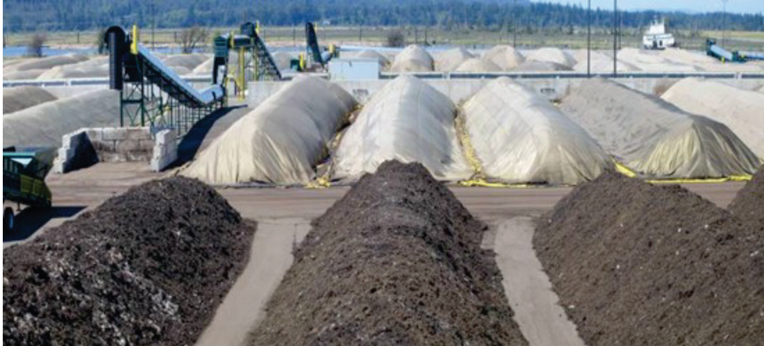
Figure 7.3 Example of a Composting Facility - Forced Aerobic Static Pile
