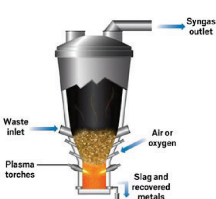
Figure 5.2 Plasma Arc Gasification Diagram
